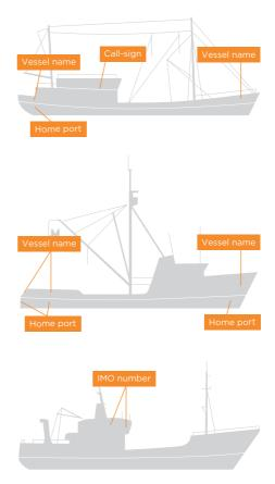
In the image below we can see vessel identity markings on all three vessels, circled in red.
