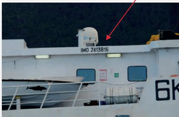
Some vessels, particularly larger ones like reefers and some purse seiners, have their IMO number visible somewhere on the hull or bridge. The IMO number is the most important vessel identifier, as it remains the same throughout a vessel's lifetime. If you can see one, it's important that you capture it on camera. In this picture (a purse seiner) you can just see the IMO number on the side of the bridge, the second picture shows it closer up.
